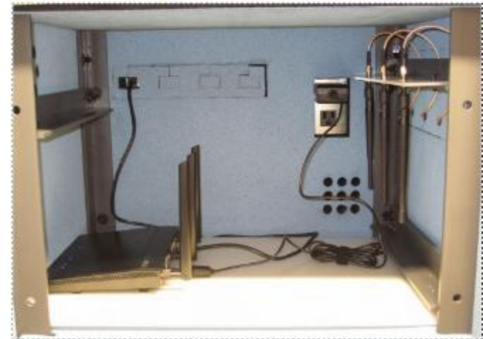
Linksys EA6000 in Upper Test Chamber - "0 degree" Position
