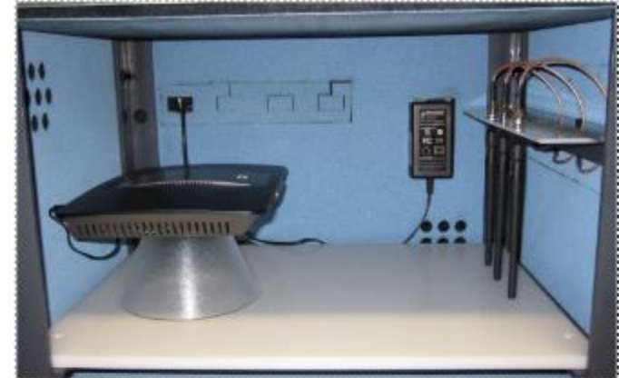
Linksys EA6000 in Upper Test Chamber - "0 degree" Position
